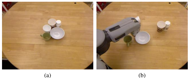
Fig. 1: Example initial cluttered scene encountered by the robot. Partial singulation result as the robot performs a pushing action.
