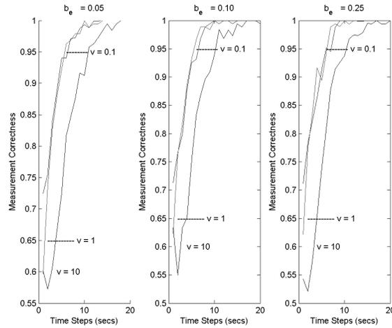
**Fig. 3** Grouping Correctness vs. Number of Samples for SBSG; left to right are for binary salt and pepper noise of 5%, 10%, and 25%; curves for 0.1, 1.0, and 10.0 variance are given in each plot.
