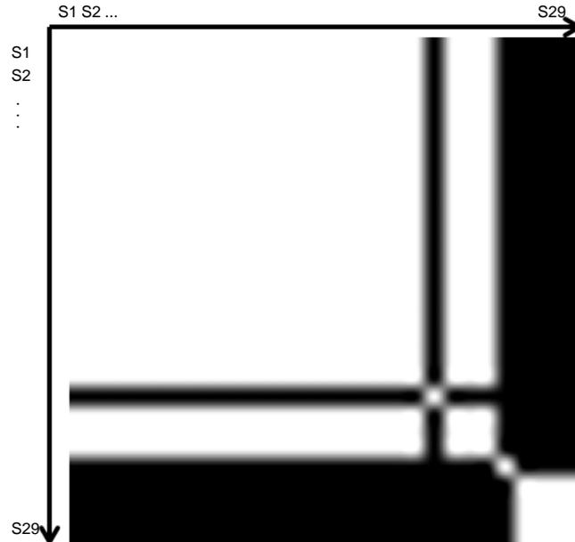
**Fig. 5** Grouping Matrix:  $29 \times 29$  binary matrix; sensors 1-24 are range sensors (sensor 21 returns constant value); 25 is energy; 26-29 are compass sensors.
