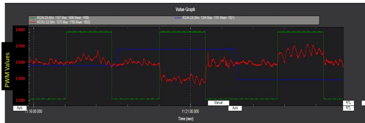
Figure 8. Autopilot Aileron Response to Varying Aileron Failure Settings.
