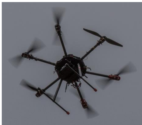
Figure 5. Tarot X6 in Hover with Right Center Motor Shut Down.
