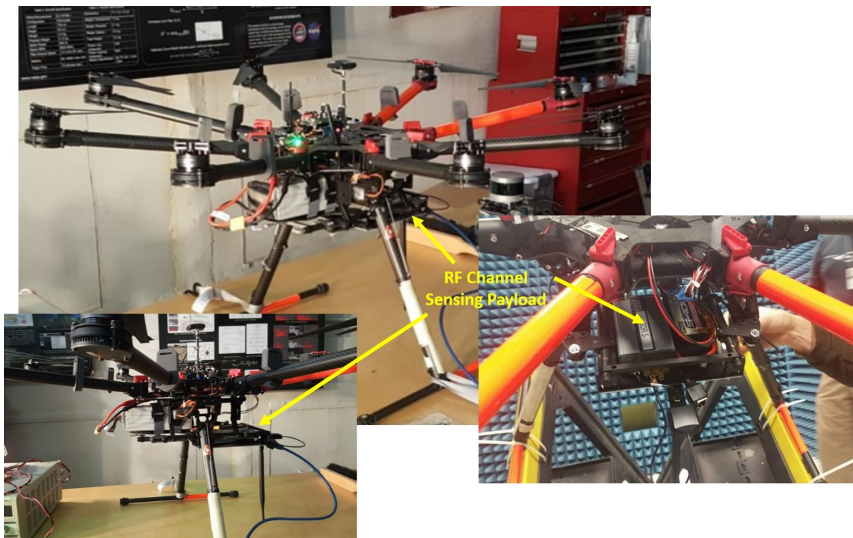
Figure 7 – Three Views of the RF Channel Sensing Payload Integration with the DJI S1000
