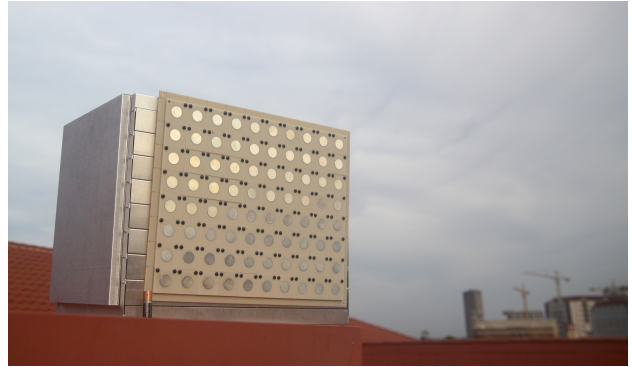
Figure 4: Complete ArgosV3 base station with 160 radios designed for 3.55 to 3.75 GHz operation. This compact cube is only 18"x14.5"x13". The plastic radome is removed to show the 80 dual-polarized antenna elements in a 10x8 configuration.
