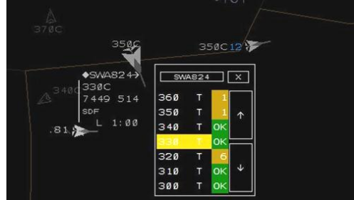
Figure 30. Altitude fly out menu with real-time conflict feedback
