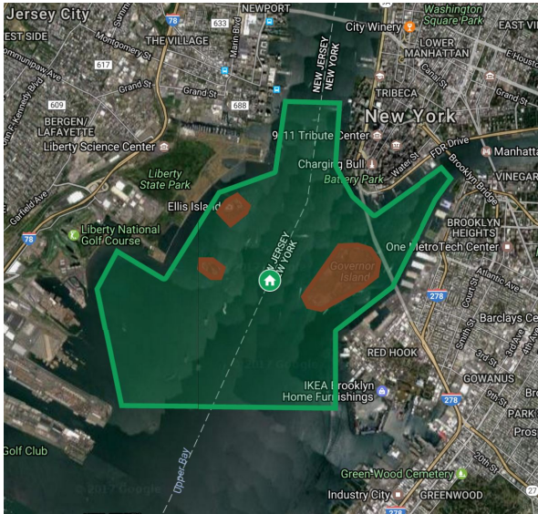
(a) Home icon - local origin. Green - keep-in geofence. Red - keep-out geofences.
