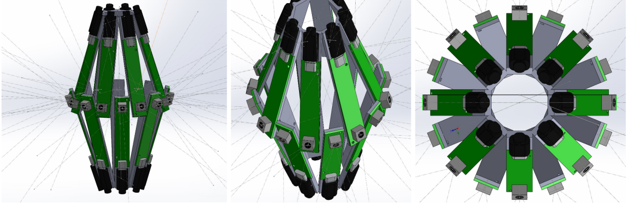
Figure 3.10: Panoramic configuration with 2 bands of See3CAM130 cameras for a larger vertical FoV
