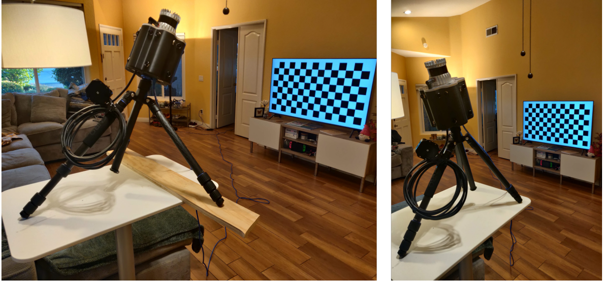
Figure 7.3: Interior, high-angle calibration procedure for the trinocular panoramic camera array
