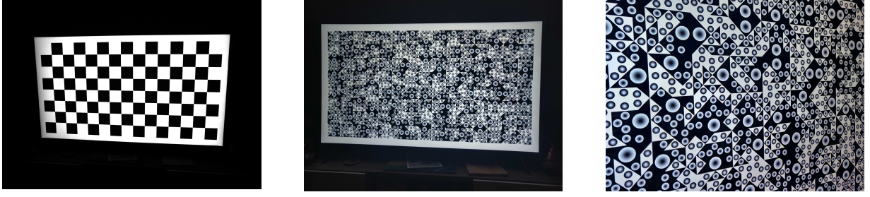
Figure 3.23: Sample calibration frames used to evaluate the checkerboard (left) and fractal (center- full, occluded- right) calibration targets.
