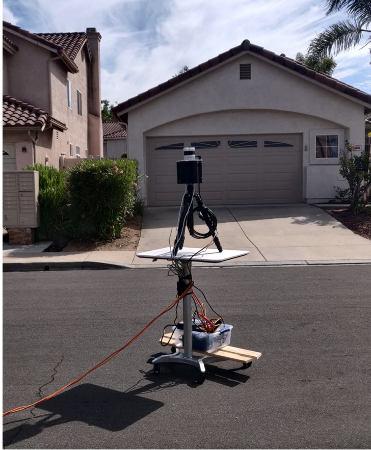
Figure 7.5: Trinocular Panoramic System Data Acquisition on an Urban Road
