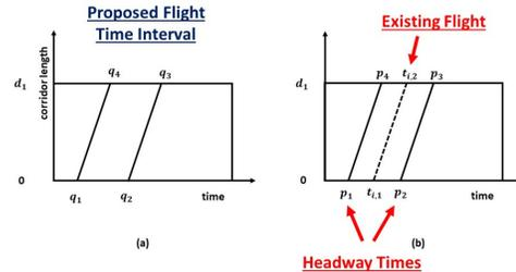
Fig. 3. The Space Time Lane Diagram. (a) Trajectories through the Lane of the Proposed Flight Earliest and Latest Possible Entry Times. (b) Trajectory of Already Scheduled Flight, and its Associated Headway Constraint Trajectories.
