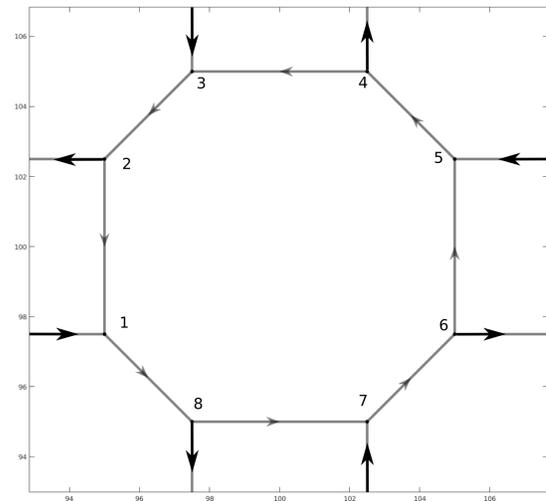
Fig. 1. An Example 4-Way Airway Roundabout.
