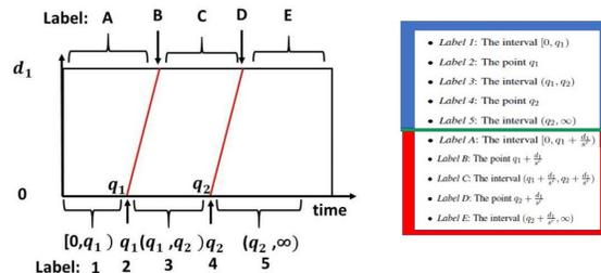
Figure 4. Space-Time Lane Diagram Labels. 1,2,3,4,5 indicate intervals and times at the entry to the lane, and A,B,C,D,E indicate times at the lane exit.
