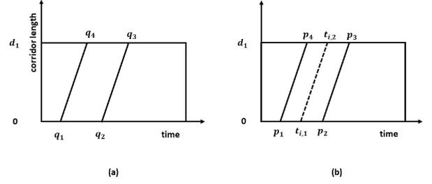
Fig. 6. Space-Time Lane Diagrams: (a) trajectory boundaries for requested launch time interval  $[q_1, q_2]$ . (b) The headway boundary trajectories for a scheduled flight which enters the lane at time  $t_{i,1}$  and exits at time  $t_{i,2}$ . The requested flight must start at some time between  $q_1$  and  $q_2$  and its path through the STLTD may not enter the  $p_1p_2p_3p_4$  parallelepiped.
