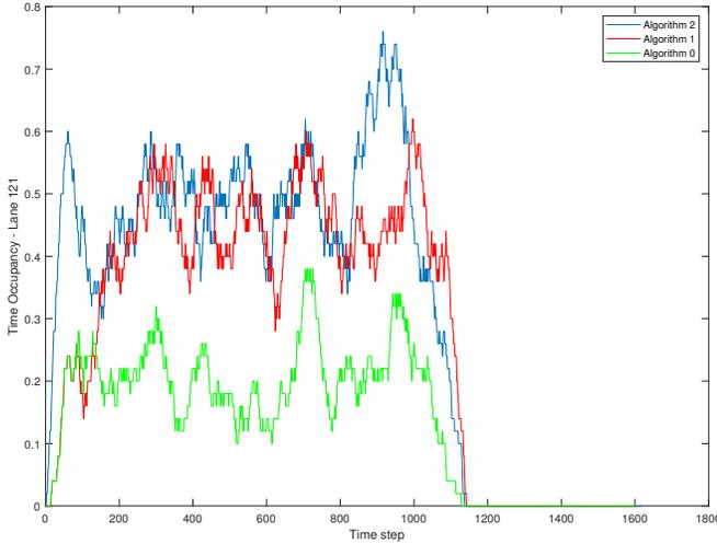
Fig. 10. Lane 121 Time Occupancy for the Three Algorithms.  $\mathcal{A}_2$  Outperforms the Other Two.
