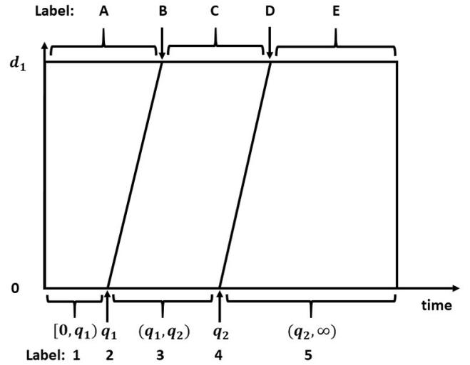
Fig. 7. Space-Time Lane Diagram Labels. 1,2,3,4,5 indicate intervals and times at the entry to the lane, and A,B,C,D,E indicate times at the lane exit.
