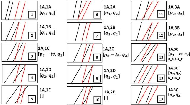
Fig. 8. Space-Time Lane Diagrams for 15 Possible Label Combinations, where  $\square$  represents the empty set. Note that Table II Provides the Complete Set of Interval Possibilities; these are the Foundation to Solve Strategic Deconfliction.
