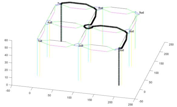
Fig. 9. 3x3 Grid Airway Layout and Example Flight Path.
