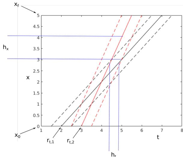
Fig. 1. Time-space diagram for two UASs in a lane. The  $x$ -axis is time and the  $y$ -axis is distance along the lane.  $h_t$  is the time headway (distance between UASs in time in lane), and  $h_x$  is the space headway (distance between UASs in lane). Note that  $h_t$  and  $h_x$  are linearly related due to the constant speed. The two trajectories in this scenario intersect at  $t = 4$  and  $x = 2$ , however they violate space-headway before then.
