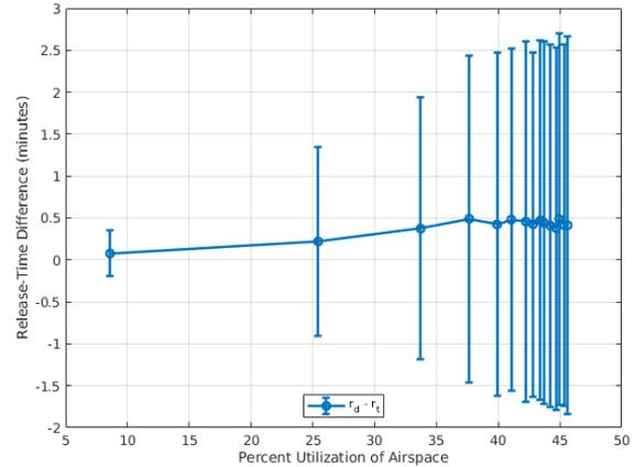
Fig. 9. Difference between desired and scheduled release time versus airspace utilization. The error bars represent the standard deviation and the round markers show the mean.
