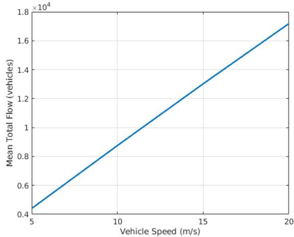
Fig. 7. Total network flow versus the speed of vehicles
