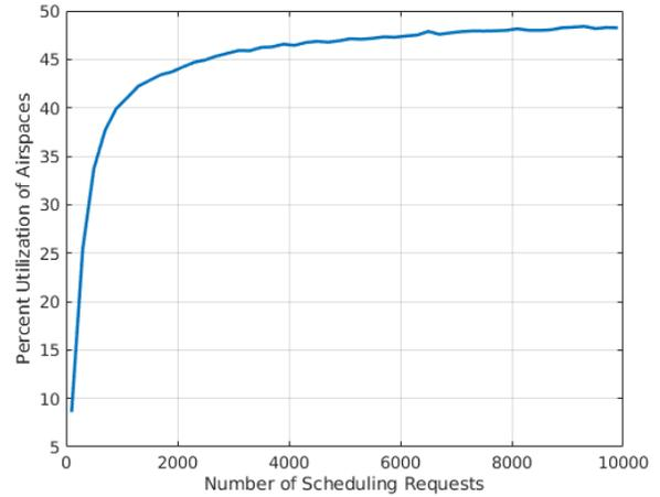
Fig. 8. Airspace utilization versus the number of scheduling requests. In this simulation the vehicle speeds were fixed to 5m/s and the headway to 25m.
