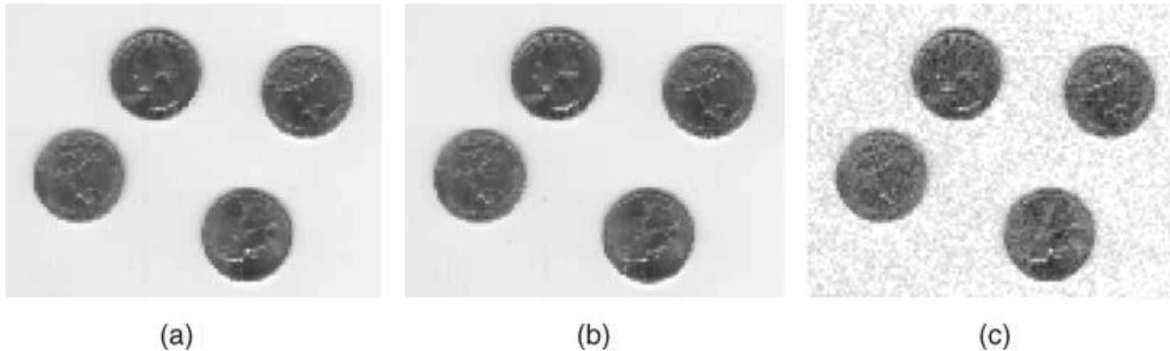
Figure 4.5 Median filter (33) applied to the (a) original, (b) 'salt and pepper' noise and (c) Gaussian noise images of Figure 4.3
