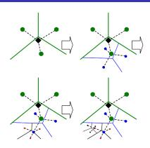
■ An illustration of the process of building the vocabulary tree. The hierarchical quantization is defined at each level by k centers (in this case k = 3 ) and their Voronoi regions.
