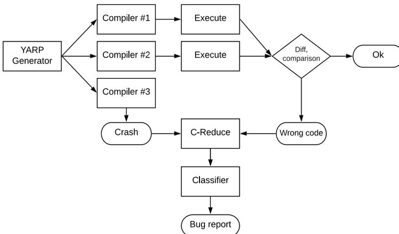
Fig. 1. Framework for differential random compiler testing
