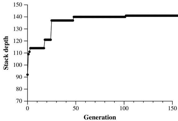
**Figure 9:** Results of using a genetic algorithm to search for interrupt schedules that maximize CntToLedsAndRfm’s use of stack memory. Although the figure stops at 150 generations, the GA was run to 500 generations without seeing further improvements.
