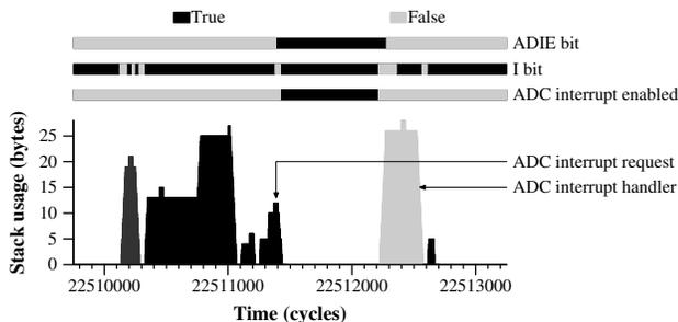
Figure 2: Visualization of about 0.5 ms of the execution of the TinyOS Oscilloscope application with RID. The ADC interrupt is enabled only after it is requested, and disabled before the first instruction of the handler executes.
