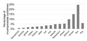
Figure 16: Percentage of incompressible cache lines across SPEC 2006 and STREAM benchmarks
