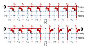
Figure 6: (a) The conventional biasing scheme during RESET phase, (b) the proposed double-sided ground biasing during RESET phase
