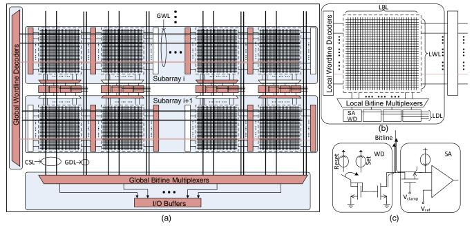
Figure 4: Modeling of ReRAM architecture in modified CACTI: (a) Schematic view of an ReRAM bank; (b) Mat organization; (c)
