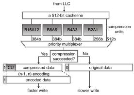
Figure 11: An overview of the compression/encoding flow
