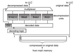
Figure 13: An overview of the decoding/decompression flow
