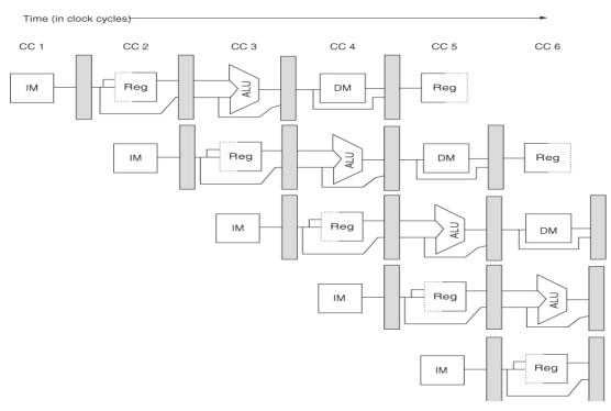
• For the following code sequence, show how the instra flow through the pipeline:
