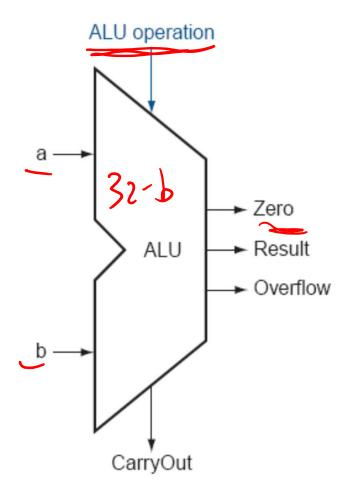
slt \$1, \$2, \$3 if k < 33Incorporating slt else 1=0 Operation Ainvert CarryIn Binvert Perform a – b and check the sign Cct for а n New signal (Less) that is zero for ALU boxes -31 1 1-31 Result b 0 • The 31<sup>st</sup> box has a unit 2 Lessin to detect overflow and sign – the sign bit Less serves as the Less signal for the 0<sup>th</sup> box Set 000. Overflow Overflow detection Source: H&P textbool
