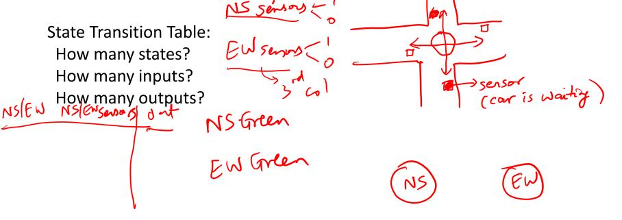
Problem description: A traffic light with only green and red; either the North-South road has green or the East-West road has green (both can't be red); there are detectors on the roads to indicate if a car is on the road; the lights are updated every 30 seconds; a light must change only if a car is waiting on the other road
