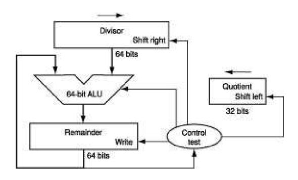
A comparison requires a subtract; the sign of the result is examined; if the result is negative, the divisor must be added back
