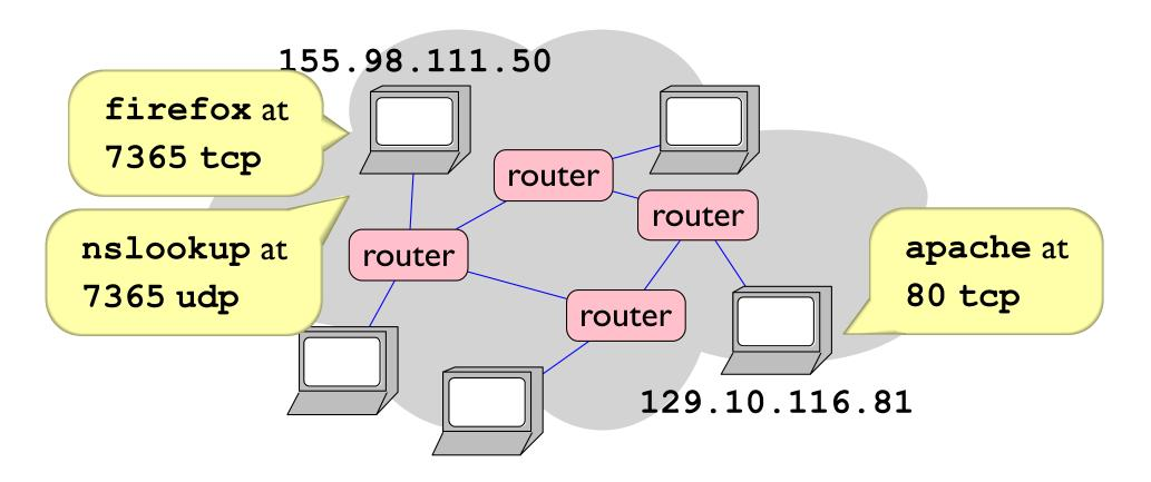
Using IP, a host is named by a 32-bit value
