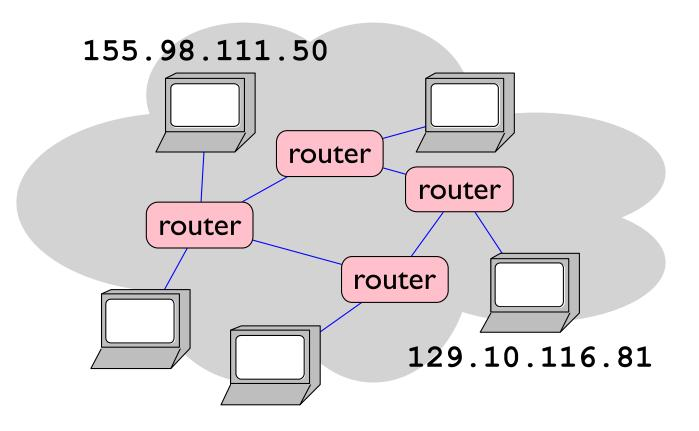
Using IP, a host is named by a 32-bit value
