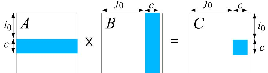
Each  $c \ge c$  block of C is computed from a  $c \ge N$  block of A and a  $N \ge c$  block of B. CS 4400—Lecture 13
