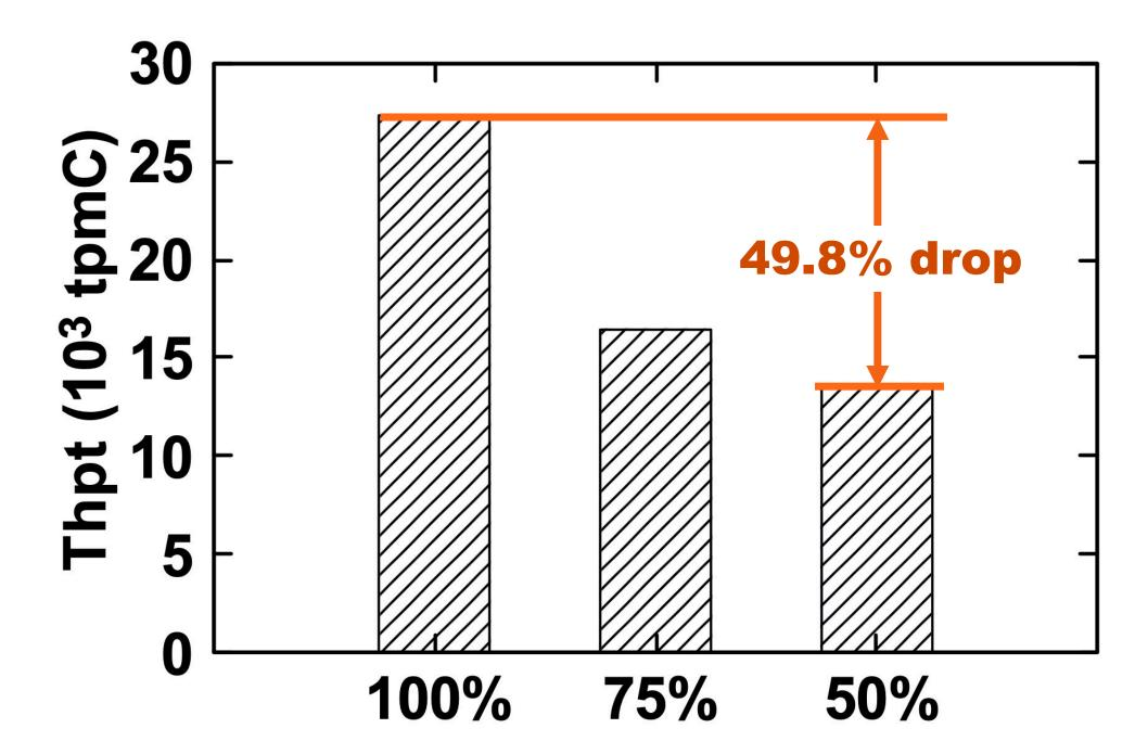
**TPC-C** Local buffer size / Data set size TPC-H Query Number **Takeaway 1:** Fast (remote) memory access advocates the co-design of database kernel and memory disaggregation.
