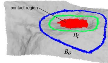
Figure 6. Estimated contact region (red) where the rock is grasped. When modeling the climbing hold, the area inside boundary  $B_i$  is unaltered. Outer boundary  $B_o$  is projected to the wall plane.
