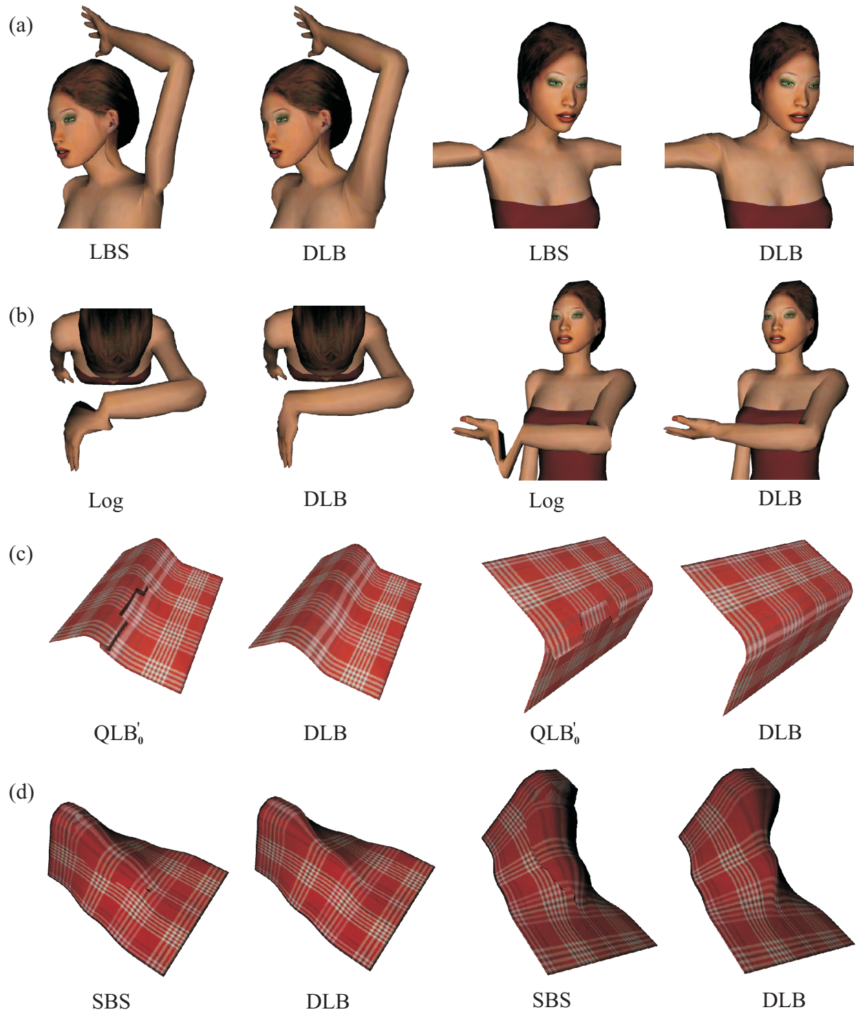
Figure 4.5: Comparison of dual quaternion skinning with (a) linear blend skinning, (b) log-matrix blending, (c) direct quaternion blending – QLB'_0 , (d) spherical blend skinning.
