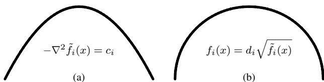
Fig. 10. Shape profiles—(a) initial parabolic profile produced by the Poisson equation, (b) spherical profile obtained by applying a cross-section function with square root.
