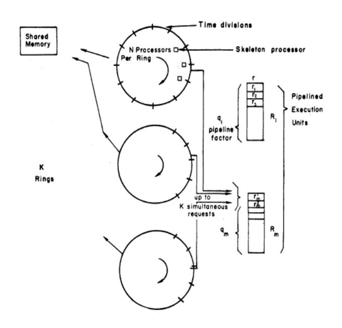
When the amount of parallelism is less than the number of processors available, a ring topology of the processor arrangement is followed which can be explained from the following diagram,
