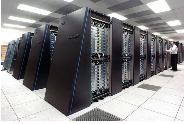
Figure 1. The Intrepid Blue Gene/P Open Science machine at Argonne with 163,840 cores, half a Petaflop (peak), consuming 1.26MW
