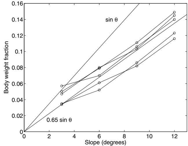
Fig. 6. Reference slope versus tether force expressed as a fraction of body weight. Slope increments are 3 degrees from 3 to 12. Data are from 5 subjects. The upper straight line is a plot of  $\sin \theta$ , where  $\theta$  is the slope in radians. The lower straight line is a plot of  $0.65 \sin \theta$ .
