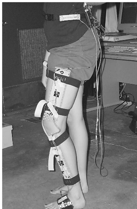
Fig. 7. Marker attachment for leg joint angle measurements.
