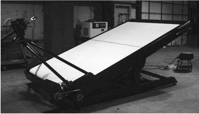
Figure 5. THE TILT CAPABILITY OF THE NEW SARCOS TREADPORT.
