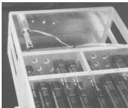
Fig. 8. Apparatus used to measure actuator force.
