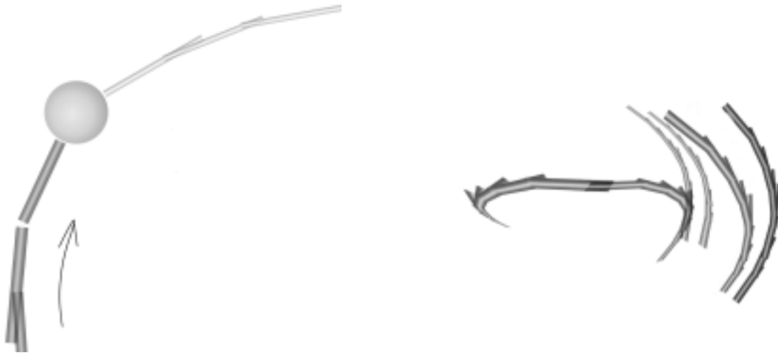
Fig 1 (left). Illustration of user interaction with flow line. The display sweeps out the path to and from the current endpoint position. The pencilled arrow indicates the direction of travel. The sphere represents the current PHANToM endpoint position; the fatter, darker lit lines are the path already taken by the user; the thin, lighter lines are the flow line leading from the current position.
