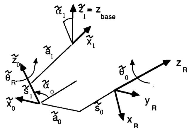
Fig. 3. The right camera axes to base D-H transformations. The first transformation locates the line of action of the right camera rotation. The second transformation locates the base coordinate  $z$ -axis, which is also the left camera axis of rotation.
