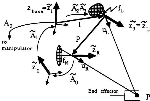
Fig. 4. A stereo camera system attached to a manipulator. *L* and *R* indicate the left and right cameras. The left and right cameras rotate about  $\tilde{z}_1$  and  $\tilde{z}_0$ , respectively.
