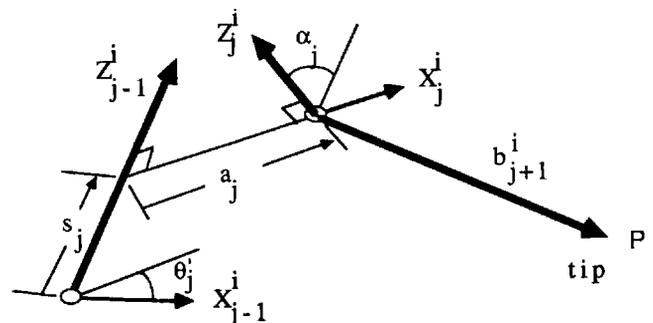
Fig. 1. Denavit-Hartenberg coordinates and tip vector  $b_j^i$ .
