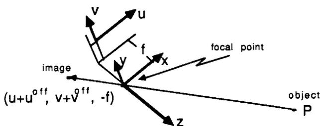
Fig. 2. The internal camera model.
