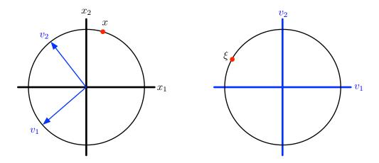
**Step 2:** ( $\eta = S\xi$ ): Note that  $\xi = (\xi_1, \xi_2)$  is still on a circle since it still has  $\|\xi\| = 1$ . The S matrix is a diagonal matrix, so it just scales the axis. Each ith axis is scaled according to  $\sigma_i$ . Specifically,  $\eta_1 = \sigma_1 \xi_1$  and  $\eta_2 = \sigma_2 \xi_2$ , where  $\xi_1$  and  $\xi_2$  are coordinates in the basis along  $v_1$  and  $v_2$ , respectively.
