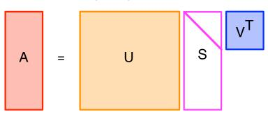
The structure that lurks beneath. The matrix S only has non-zero elements along its diagonal. So  $S_{i,j} = 0$  if  $i \neq j$ . The remaining values  $\sigma_1 = S_{1,1}, \sigma_2 = S_{2,2}, \ldots, \sigma_r = S_{r,r}$  are known as the *singular values*. They have the property that
