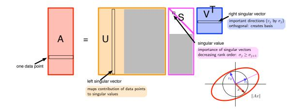
**Tracing the path of a vector.** To illustrate what this decomposition demonstrates, a useful exercise is to trace what happens to a vector  $x \in \mathbb{R}^d$  as it is left-multiplied by A, that is  $Ax = USV^T x$ .
