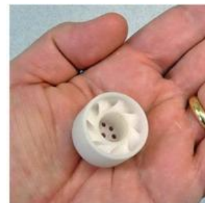
1" burner (5 kW, 17 KBtu/hr)
