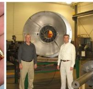
28" burner (44 MW, 150 MBtu/hr)
