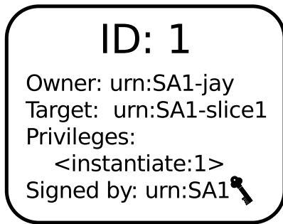
Figure 2. Example credential, showing target, owner, a set of permissions, and a signature. Note that the URNs in this figure are abbreviated.
