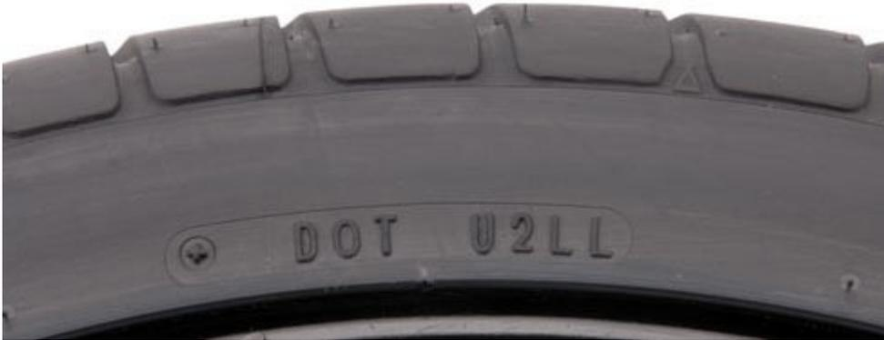
The use of a partial Tire Identification Number on the one sidewall (shown above) reduces the risk of injury to the mold technician that would have to install the weekly date code on the top sidewall portion of a hot tire mold.
