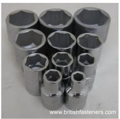
heads, and hence wrench sizes. The most commonly seen threads are 1/4 x 26 BS, 5/16 x 22 BS, 3/8 x 20 BS, 7/16 x 18 BS, 1/2 x 16 BS, and 9/16 x 16 BS. Wrenches labeled BS come in the these sizes, labeled by bolt diameter. Hence for the bolt sizes listed above, we use BS wrenches labeled 1/4, 5/16, 3/8, 7/16, 1/2, and 9/16 inch, respectively.
