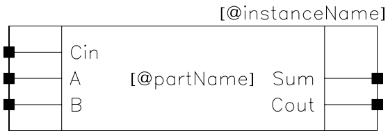
Figure 3.8: A simple symbol for the FullAdder circuit
