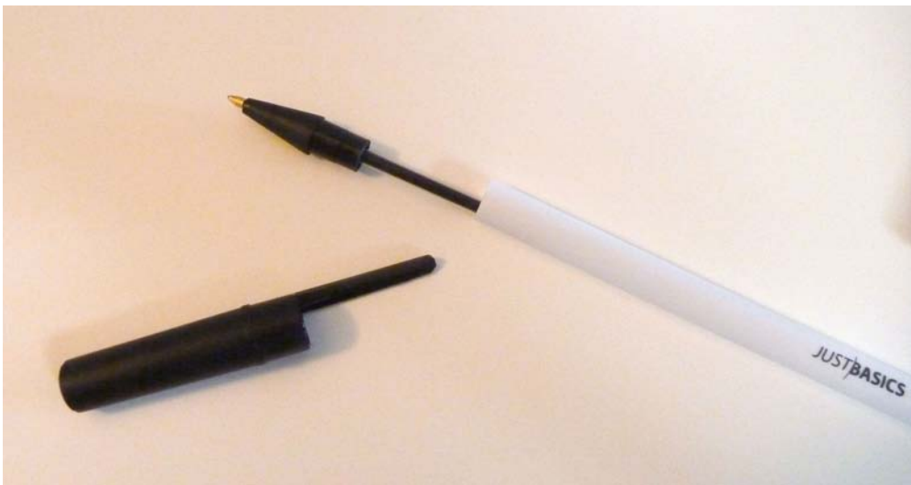
Figure 16: First I'll take the pen apart to get at the thinner pen insert in the center.
