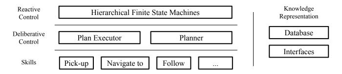
Figure 2: Functional components of our LAAIR implementation for HSR.
