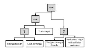
Figure 3: Behavior tree for person following skill. Arrows indicate sequence nodes and question marks indicate fallback nodes.
