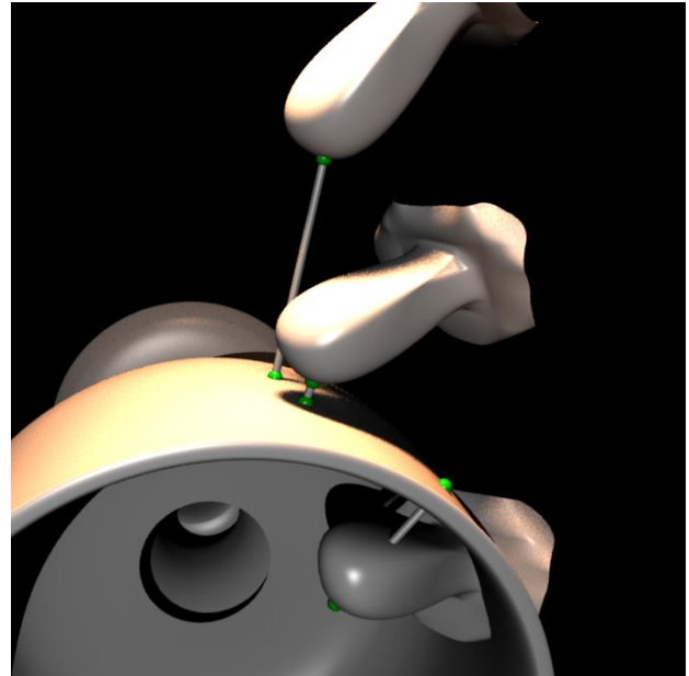
Figure 2: Virtual proxies are important in the penetrating case. The maximal distance is required by the haptics tracing algorithm. Global solution discontinuities such as “chopping though” an object are not desirable. Because the velocity formulation (shown) is the “most local,” it is the method of choice for the penetrating case.
