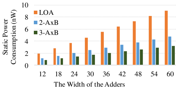
Figure 12: Comparing static power consumption of several multi-bit adders comprising 2 and 3-AxBs with LOA.
