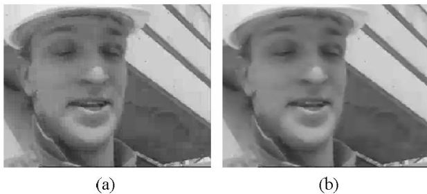
Figure 8. Applying the 2-D deblocking filter to CIF foreman test sequence. (a) not-filtered sequence; (b) filtered sequence.
