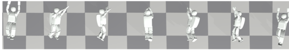
Figure 2.3: A kinematic rolling motion is retargeted to a physics based Asimo-like character [15]. Used with permission.
