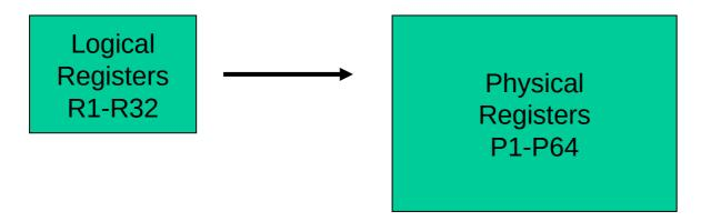
At the start, R1-R32 can be found in P1-P32 Instructions stop entering the pipeline when P64 is assigned
