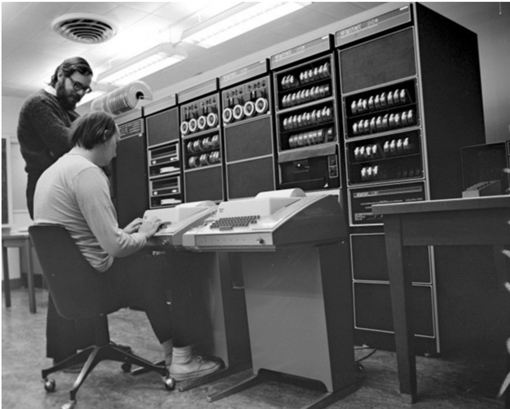
Ken Thompson (sitting) and Dennis Ritchie (standing) are working together on a PDP-11 (around 1970). They are using Teletype Model 33 terminals.
