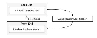
Figure 5.1. Debugger construction process
