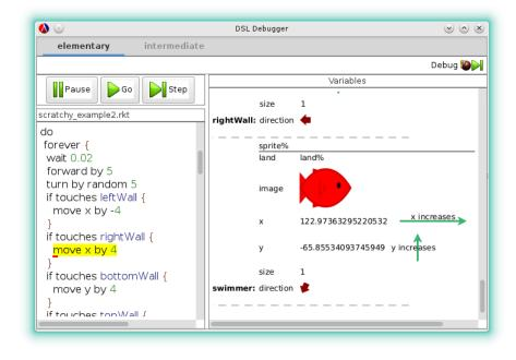
Figure 6.7. Scratchy debugger interface after second step
