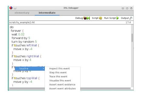
Figure 6.3. Scratchy debugger interface in an intermediate mode
