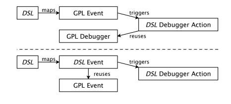
**Figure 4.2**. A comparison of the traditional approach (top) and my approach (bottom) to DSL debugger construction
