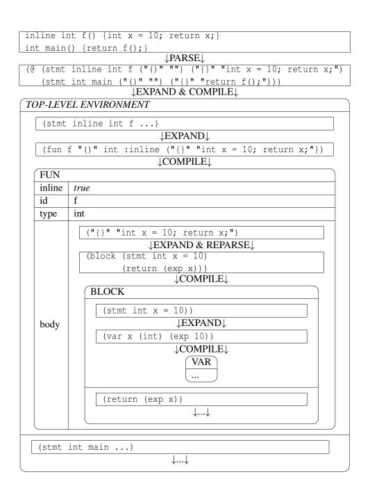
Figure 4.1. How ZL compiles a simple program. The body of f is reparsed and expanded as it is being compiled.
